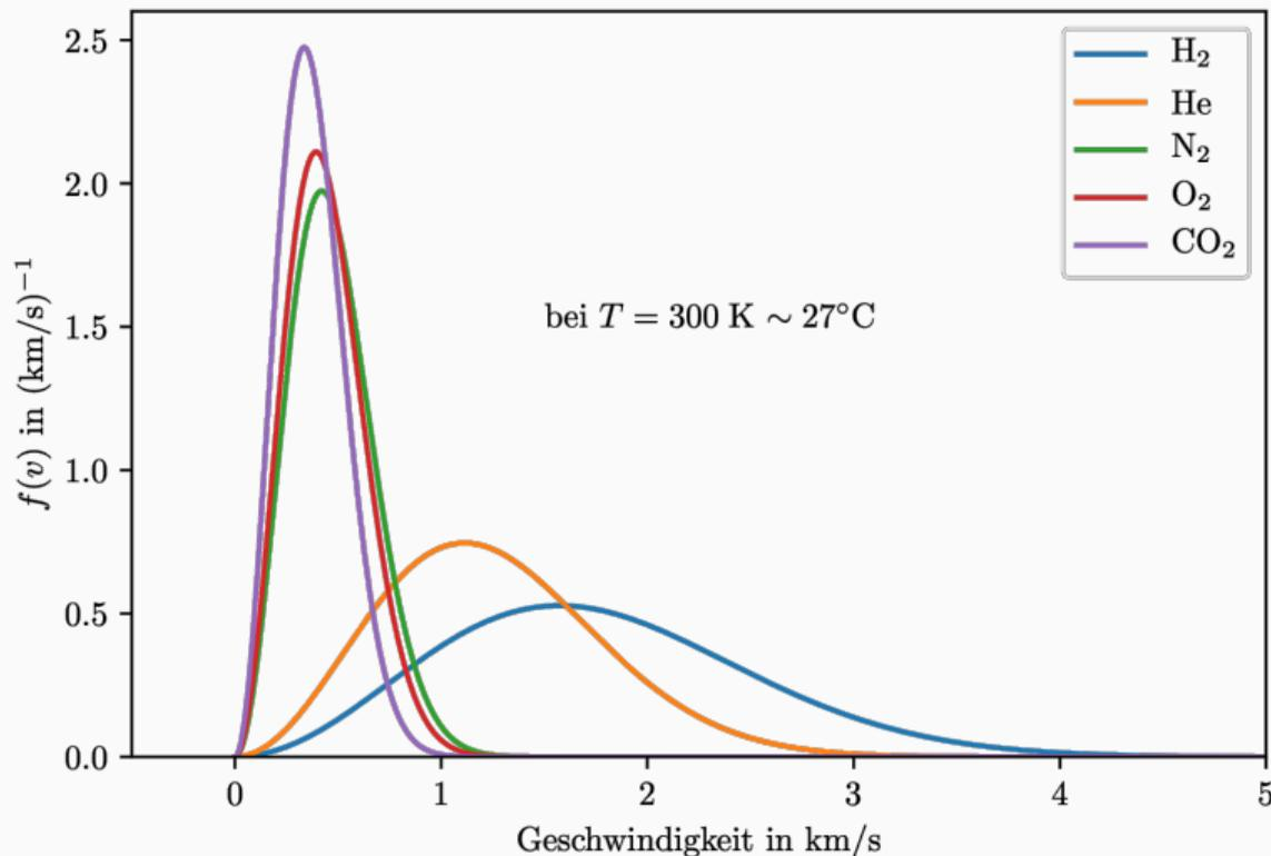
$$v_{th} = \bar{v} = \sqrt{\frac{8k_B T}{\pi m}}$$
