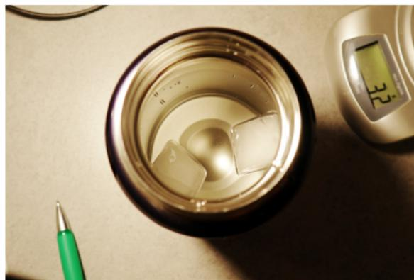
$$m_W = 475 \text{ g}, m_E = 22 \text{ g}, \vartheta_W = 23.4^\circ\text{C}, \vartheta_M = 19.5^\circ\text{C}$$
