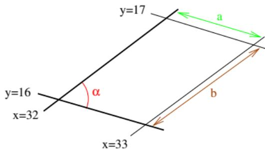
Assume an isometric view (straight down onto the plane): read off 3 parameters!
